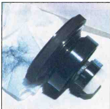
Figure 3. Clutch tire after roughening with fine emery cloth. Tissue shows tire residue.
